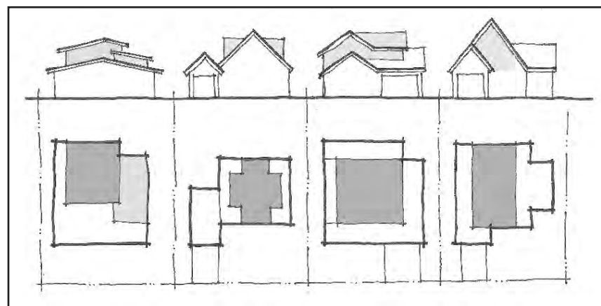
Second story additions held toward the center and stepped back from the footprint of the original building provide appropriate scale and mass. This diagram shows the additions in both elevation and plan. Shaded areas are new.
